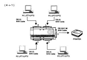
Fig. A 4-IN- 1 -OUT configuration
